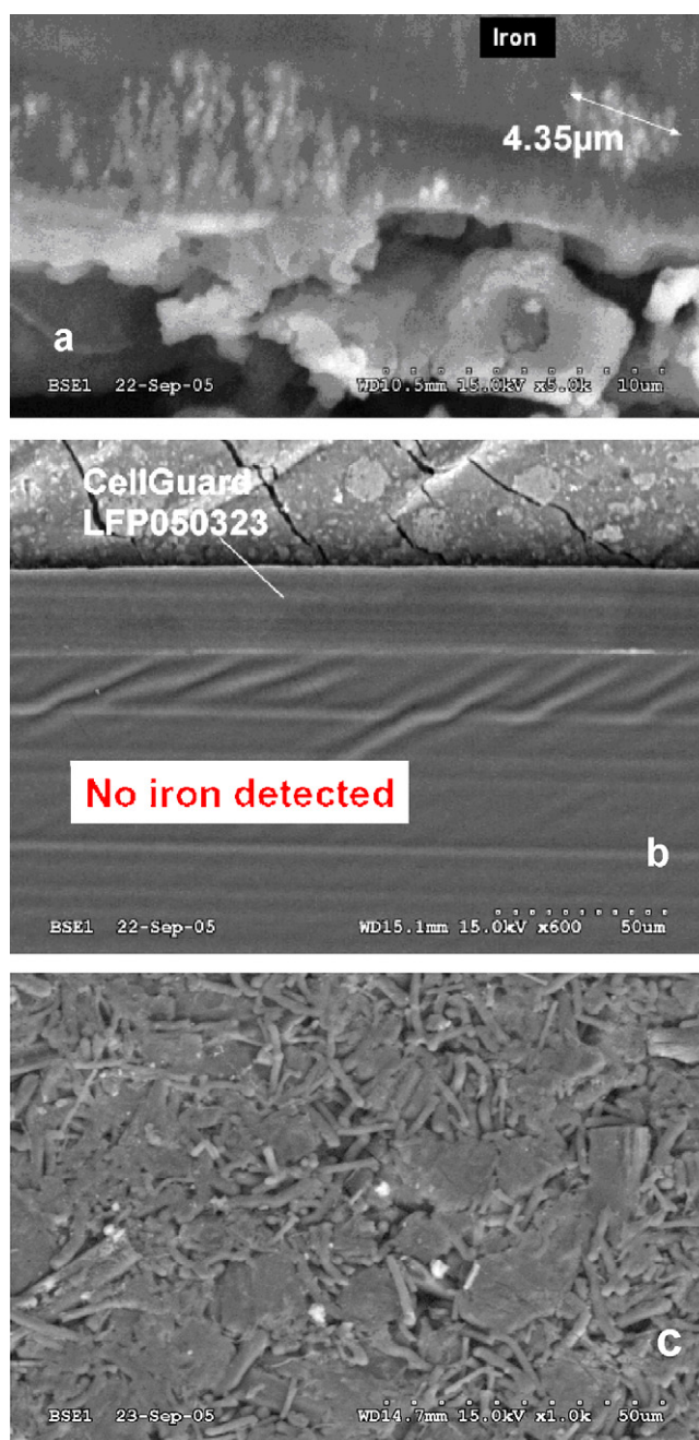
Fig. 3. Post-mortem SEM images of the detection of iron species at the separator/lithium interface. (a) Image showing the formation of iron islands at the interface with an earlier generation of \text{LiFePO}_4 . (b) No iron was detected at the surface of lithium foil with the optimized \text{LiFePO}_4 . (c) Li-ion graphite electrode after 200 cycles does not show the presence of iron particle.
